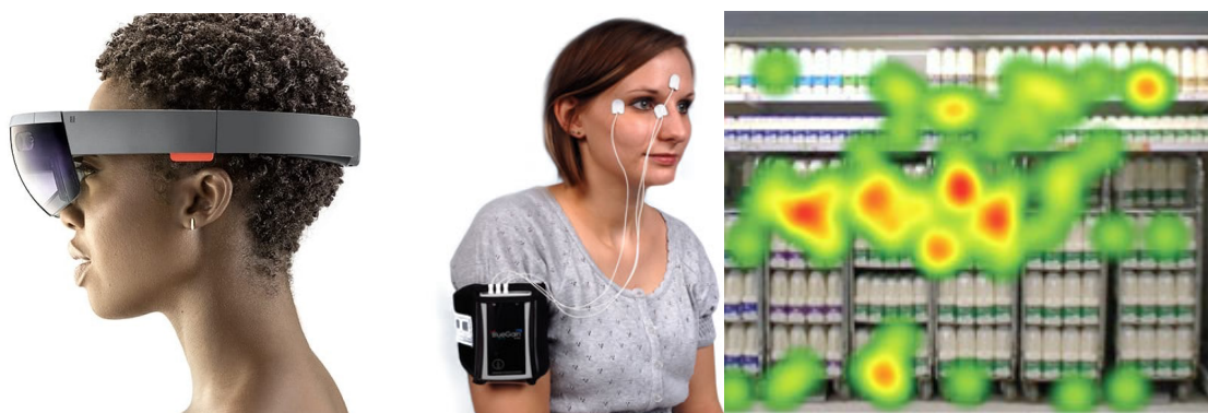
Figure 1: Left: see-through display in Microsoft HoloLens ( https://www.microsoft.com/de-de/hololens ). Middle: Recording eye movements by means of electrooculography (Cambridge Res. Systems). Right: Heat map of eye fixations.
