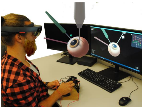
Figure 2: Microsurgical simulator for testing ergonomics design of microsurgical instrumentation. Microsoft's HoloLens is used as display technology. Continuous tracking and evaluation of micro-manipulations by means of an optical IR system.
