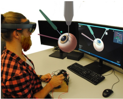
Figure 1: Microsurgical simulator for training the procedure of peeling the internal limiting membrane of the retina. Includes an intelligent tutoring system improving efficiency of training. Microsoft's HoloLens is used as display technology. Continuous tracking and evaluation of micro-manipulations by means of an optical IR system.
