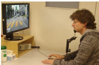
Figure 1: Visual attention test set up: Participants position their head into a rest and observe the test images presented on the monitor.
