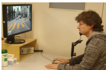
Figure 1: Visual attention test set up: Participants position their head into a rest and observe the test images presented on the monitor.
